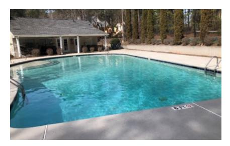
There are several types of plaster that can be used for a pool. All of them use white Portland cement, so the difference is other components. The first type is standard plaster that adds fine marble aggregate to make the plaster with a life of about nine years. The second type is an upgrade that uses fine quartz aggregate instead of marble that is about 20% more expensive but lasts about eleven years. The third type is Pebble Tec, an exposed aggregate surface where
